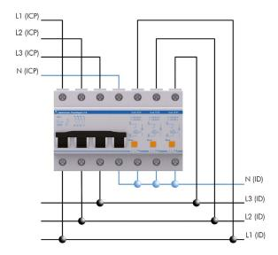
**IGA TEST** series protectors cut off the power supply when they detect a permanent overvoltage (for example, a fault in the neutral), thus protecting the equipment installed downstream.
