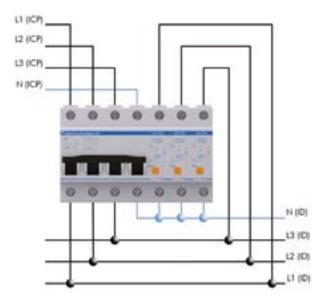
**IGA TEST PLUS** series protectors cut off the power supply when they detect a permanent overvoltage or undervoltage, (for example, a fault in the neutral), thus protecting the equipment installed downstream.
