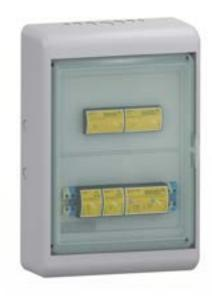
For all of the protectors to work, they must be separated by at least 10 metres of cable or a decoupling inductor which also withstands the line operating current. The complete ATBARRIER systems have been designed in this way.
