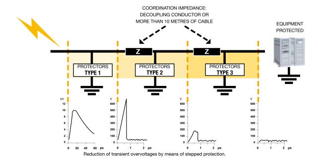
Many protectors are formed by the combination of these elements or by several of them coordinated in a single device. Decoupling elements are normally resistances or inductors with very low impedances given that, as they are in series with the line, current continuously flows through them. If impedances were high, they would cause unnecessary losses and consumptions.
