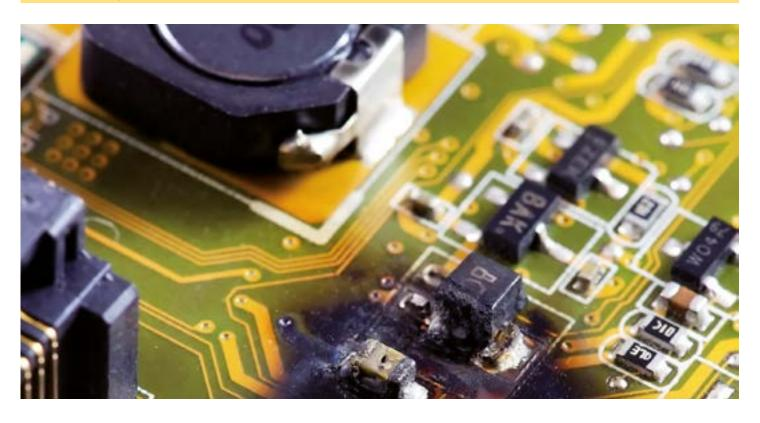
The most typical transient overvoltages are due to switching operations of machinery. However, the most destructive ones are due to atmospheric discharges.
