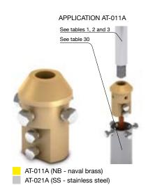
Suitable for fixing the lightning rod in the mast (table 26) with internal conductor (tape, cable or round) connection. Air termination rod as AT-121A (table 3) or AT-114A (table 7) can be fixed in AT-161A.
