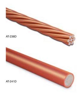
Copper-clad aluminium conductors (Cu 15%) maintain the electrical characteristics of copper conductors but with a lower cost. Installation with this material is easier than using copper-steel due to its high malleability.
