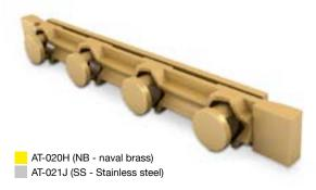
AT-020H and AT-021J enable the down-conductor of the lightning protection system to disconnect from the earth electrode in order to correctly measure the earth resistance. They are ready to be fixed to the AT-010H earth pit. Up to 4 copper cables or round bars and 3 tapes can be connected.
