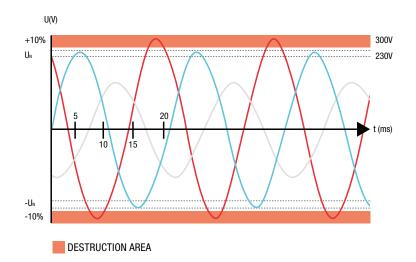
In order to protect equipments against the effects that these overvoltages may cause, Power Frequency Overvoltage Protectors (POP) must be installed, which disconnect the installation from the power supply network.
