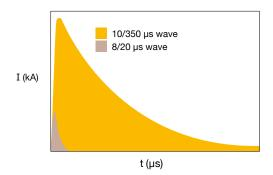
Impulse current waves applied to overvoltage protectors in order to check their characteristics. The area of each curve in this graph shows the specific energy applied.
