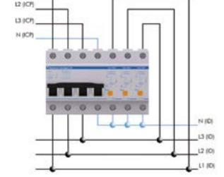
**IGA TEST** series protectors cut off the power supply when they detect a permanent overvoltage (for example, a fault in the neutral), thus protecting the equipment installed downstream.
