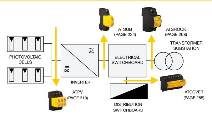
The electrical installation should be protected as follows:
