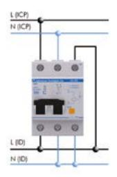
**IGA TEST** protectors actuate when they detect a permanent overvoltage (for example, a fault in the neutral), protecting the equipment installed downstream.
