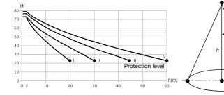
Franklin rods should be placed on the higher and most vulnerable places (corners, overhangs, etc.), as shown in the figure:
